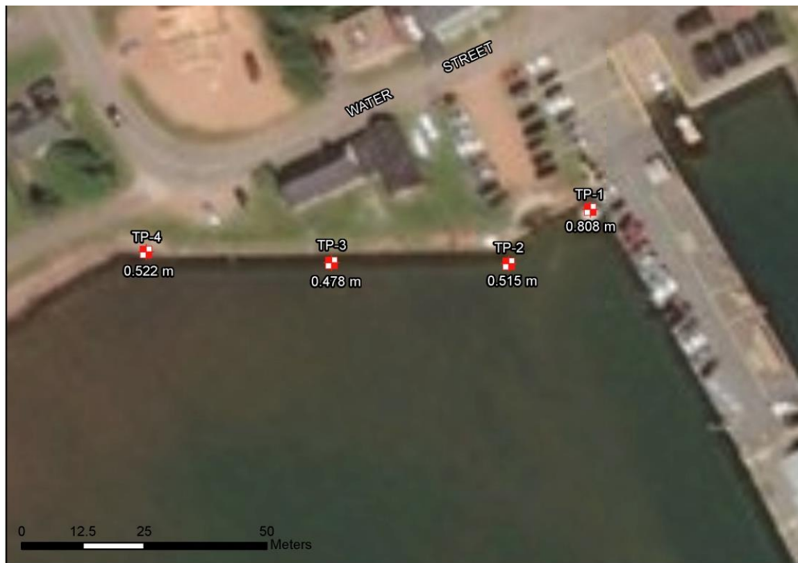
Figure 18 – The location of the four test pits, and the height above Mean Low Water of each, at the Community of Victoria Seawall site.
