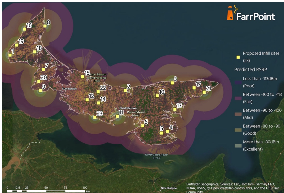
Figure 19: Infill Analysis Results – New Tower Locations and Predicted Coverage
