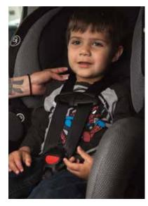
You should not be able to hold a pinch of the harness together at the shoulder.
