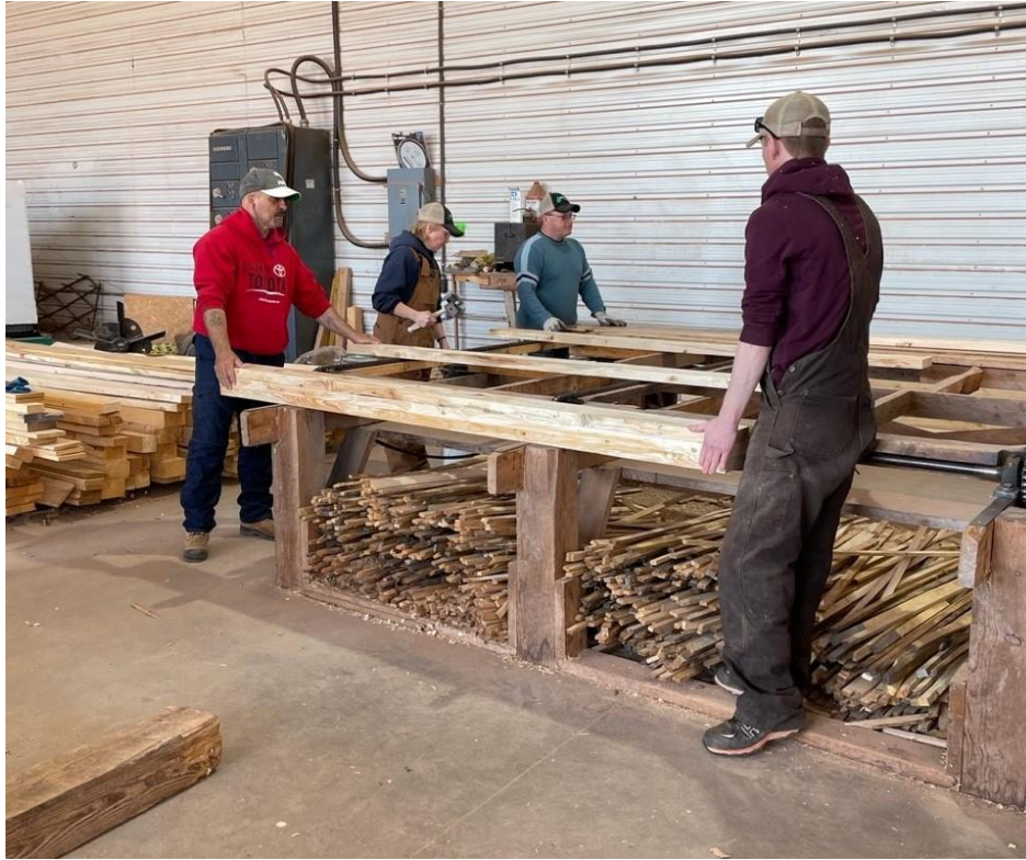
Kelley Wood grading 2x6 lumber as it comes from the planer – Betts Mill, Glenwood May 12, 2023
