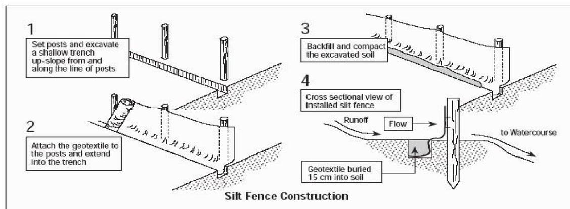
**WOVEN AND NON-WOVEN SYNTHETIC FABRICS** are available for use as silt fences. Fences are used for controlling sheet run-off, on relatively low slopes or to delineate the downslope edge of a construction site. The fabric is erected, to a height no greater than 0.9 meters above ground level, using wooden or steel posts. Reinforcement of the fabric may be necessary. The bottom of the fabric should be buried in a trench and backfilled.
