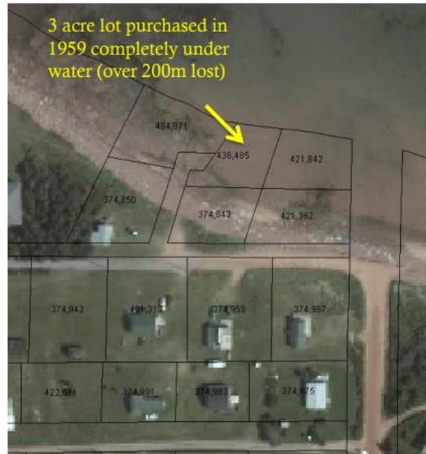
Figure 28. Photo exhibiting coastal erosion within the last 80 years on PEI [8].
