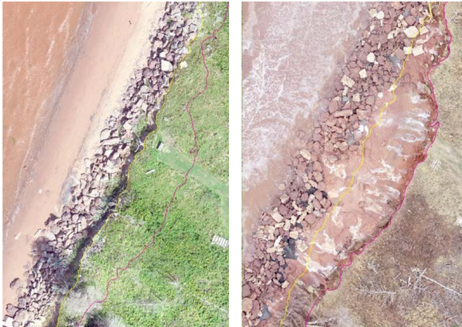
Fig 28. Section of Miminegash coastline from August (left) and November (right) RPAS flights showing coastal changes
