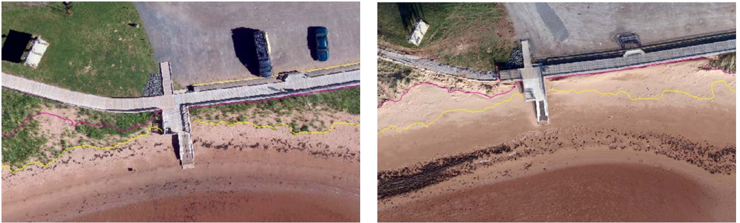
Fig 36. Section of Souris coastline from July (left) and November (right) RPAS flights showing erosion on either side of stairs
