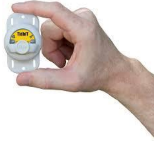
Figure 11. Hobo Tibit Temperature Devices (MX 2203).
